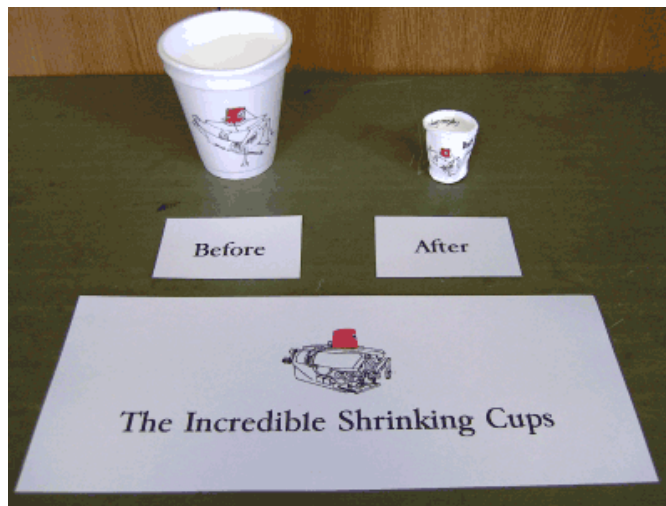
figure 3: This is what happens to a styrofoam cup taken 300-400 m underwater. Styrofoam is a hydrocarbon polymer made up of 95 % air. photo by Captain Gary Chiljean © Nautical Vows
