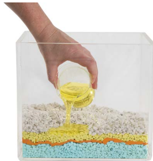
Figure 2.8 Addition of confining layer to model Paul Ricketts
