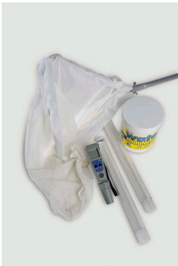
Figure 4.7 LaMotte water monitoring kit Paul Ricketts
