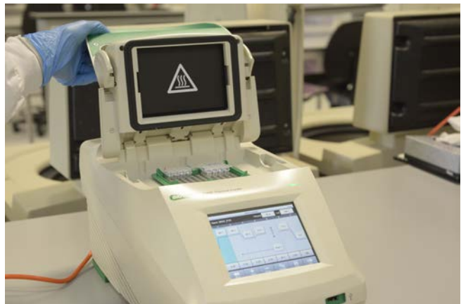
Thermocycler: repeated cooling and heating of DNA samples amplifies DNA.
