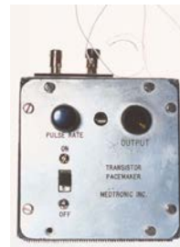
Prototype external pacemaker (1957)
