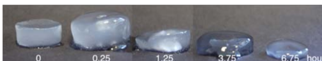
Figure 5: Degradation of a peptide-crosslinked pHEMA sample under the action of the enzyme papain in a laboratory test over about 7 hours. (photo courtesy Dr Ylenia Casadio)
