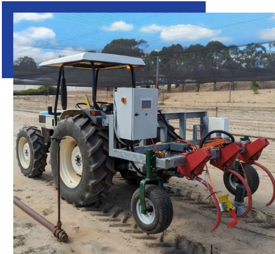
Engineering 3-tyne test rig at Shenton Park Field Station.
