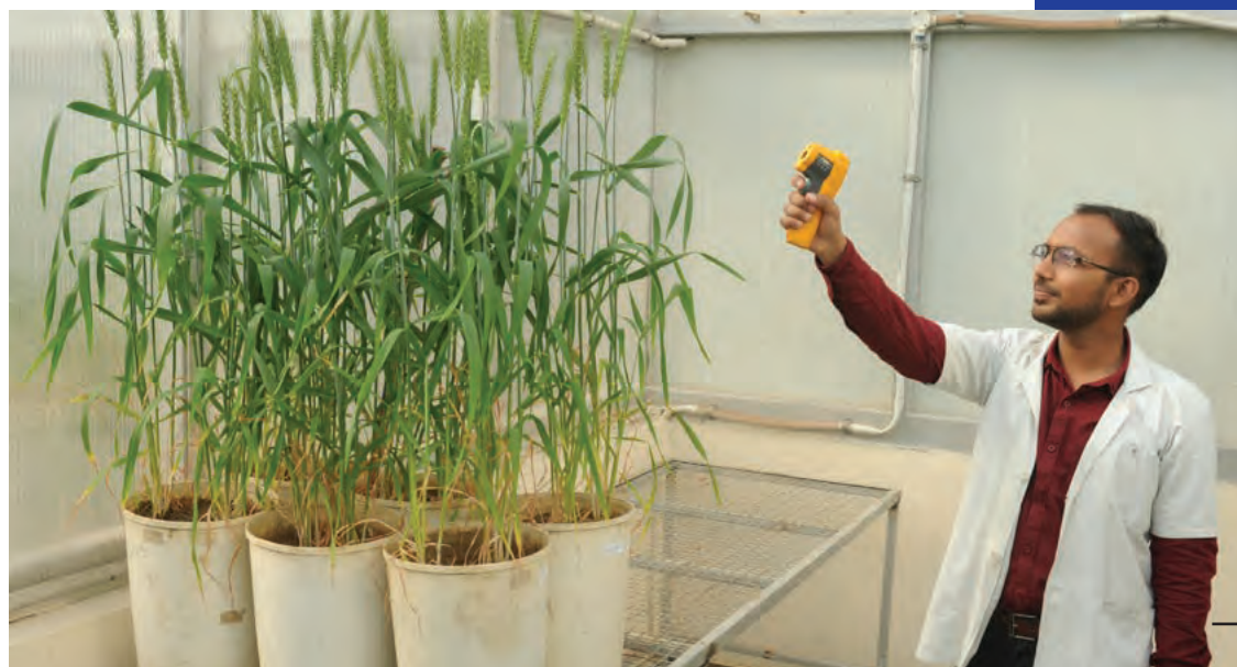
Agyeya Pratap during his first stress trial recording leaf, spike and canopy temperature using infrared temperature sensor at IARI.
