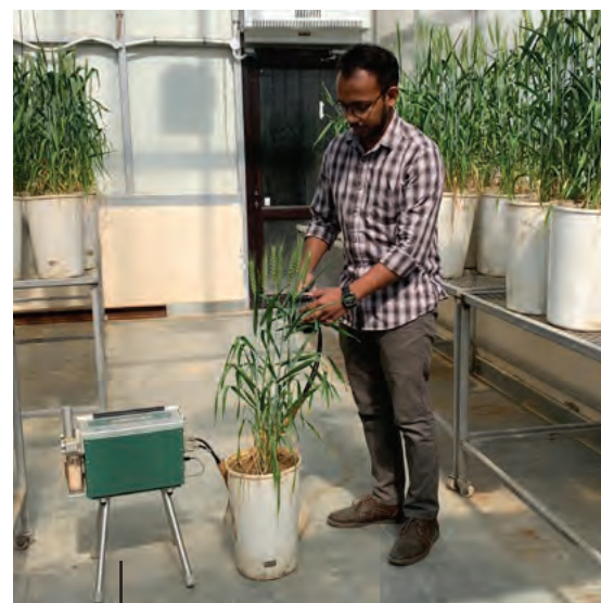
Recording leaf gas exchange using infrared gas analyser.
