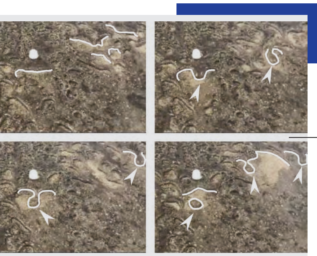
Progression through time showing movement of water across the surface leaving dry soil below and carrying soil particles on the outside of the water body. White point is a surface position marker, white lines and arrows show the water front moving as it moves across the surface. Photos taken in sequence on the 6° slope with untreated soil on the first rainfall event.
