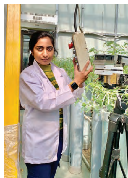
Remote-control being used by Ms Reddy to lift the PVC-tubes, using custom-designed gantry hoist to decide the daily transpiration of chickpea plants in drought experimental setup.
