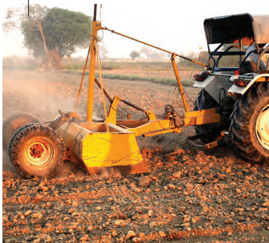
A Landking laser land leveller pictured in a field in India.
