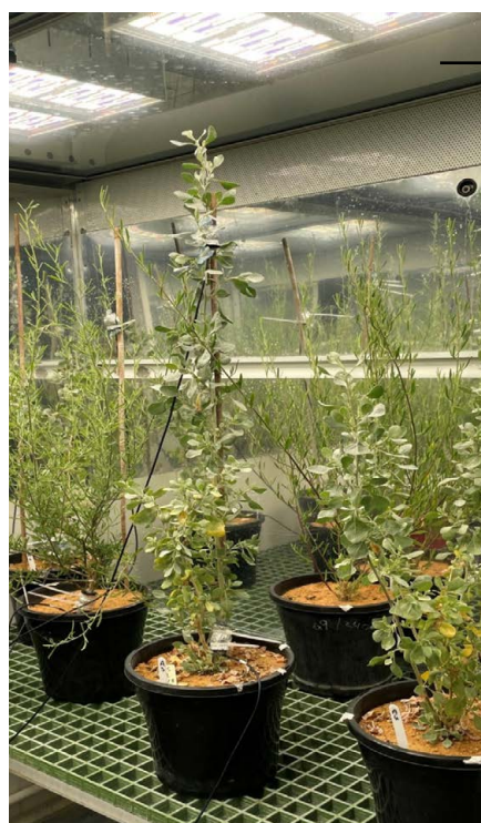
Monitoring plant water use in a controlled environment using custom-built sap flow sensors on the stem top and base.
