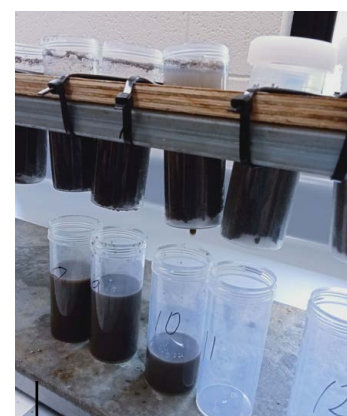
Leaching apparatus collecting leachate from soil columns to assess nitrogen losses. Experiment was performed by Anna Osmond during February-March 2025.
