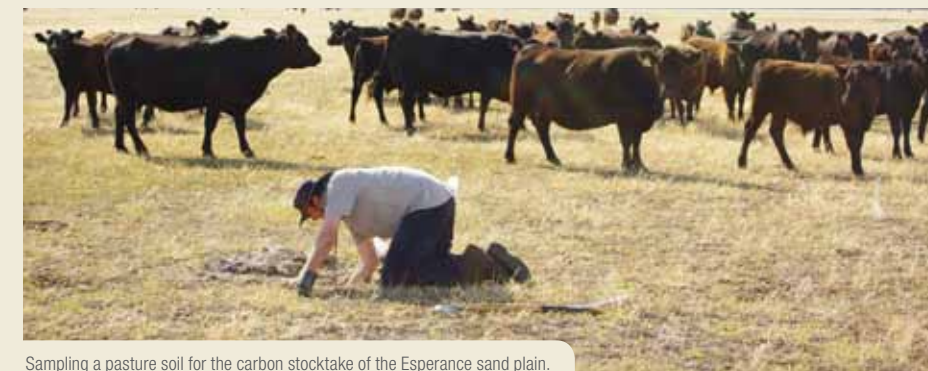
Sampling a pasture soil for the carbon stocktake of the Esperance sand plain.
