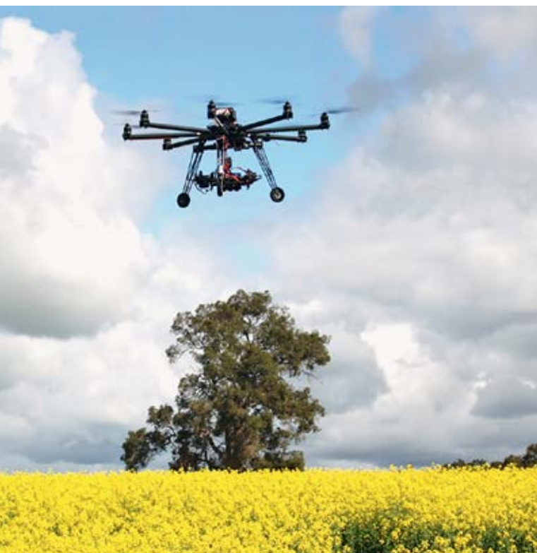
Eight-rotor unmanned aerial vehicle acquiring multispectral images of canola canopy.
