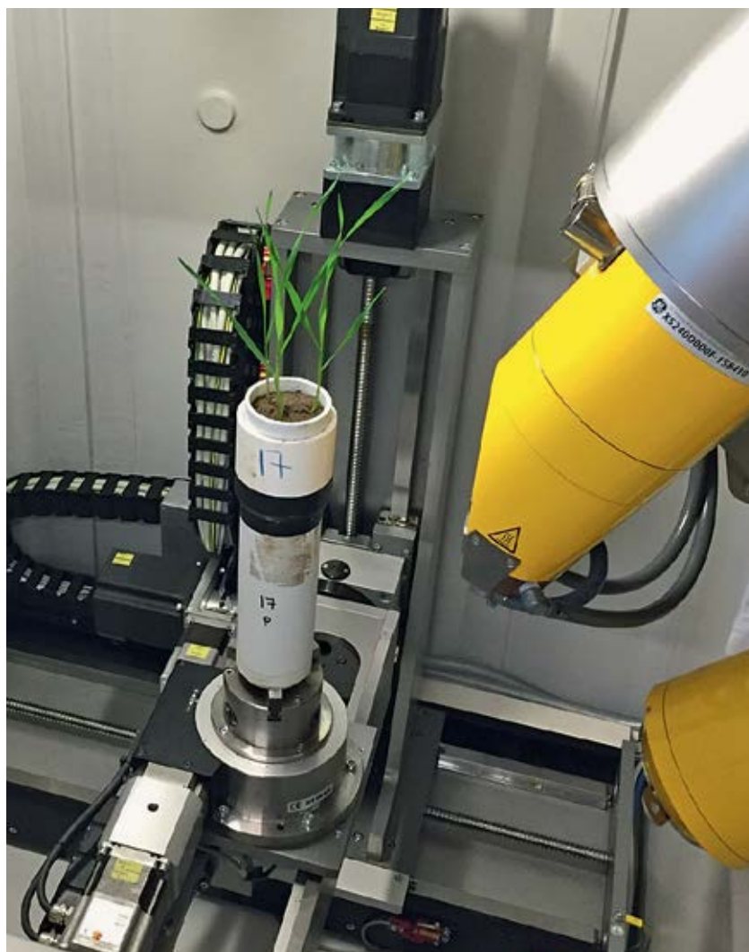
Soil core being scanned at the UNE cat scanning facility. Photo: Richard Flavel
