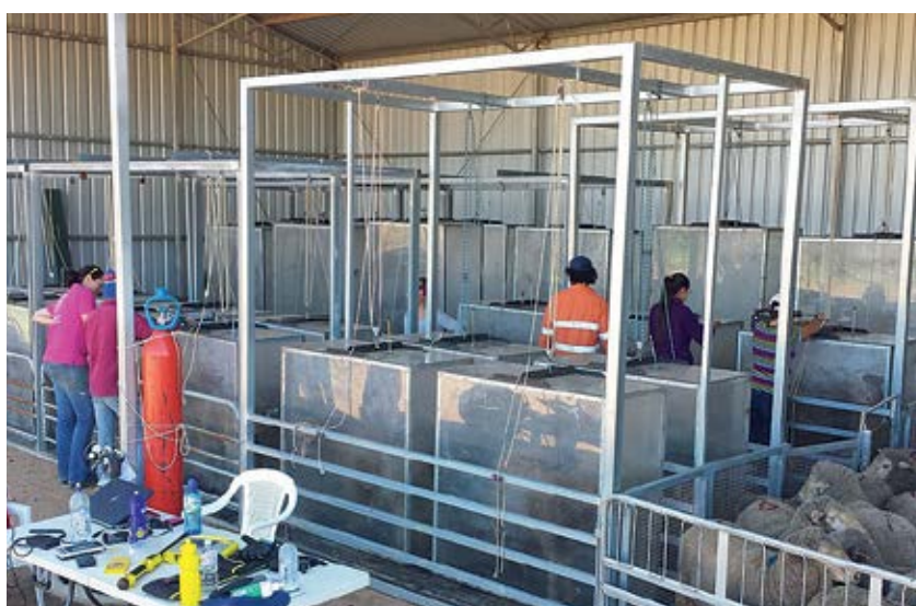
Portable accumulation chambers and a flame ionisation detector were used to measure 1-hour of methane from each sheep.
