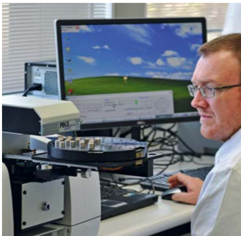
Richard Bowles (UWA) doing Mid-Infrared spectroscopy (MIR) scanning of soil samples at DAFWA
