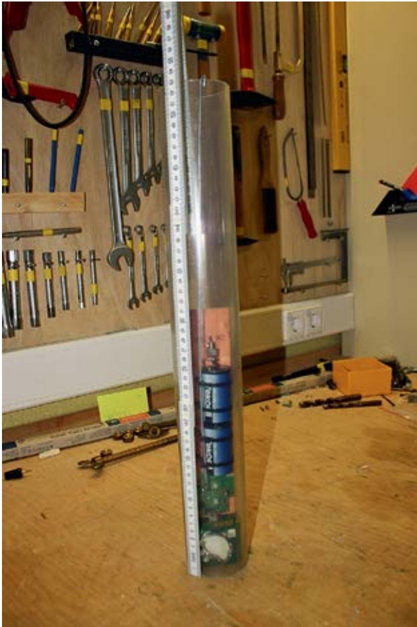
Underground Wireless Network Sensor
