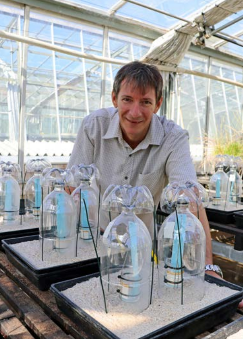
Research Officer Paul Damon testing the semi-open passive chamber method before commencing experiments.
