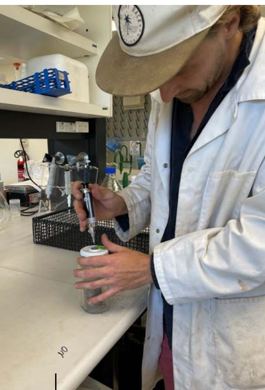
Collecting headspace gas to measure carbon dioxide production (microbial respiration).
