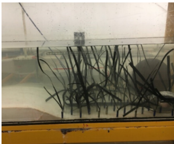
Image: Artificial Seagrass mats (ASMs) are efficient in capturing sediments and this efficiency increases with mat shoot density. This image shows the start of the test. Image courtesy of Hannah Dawn.
