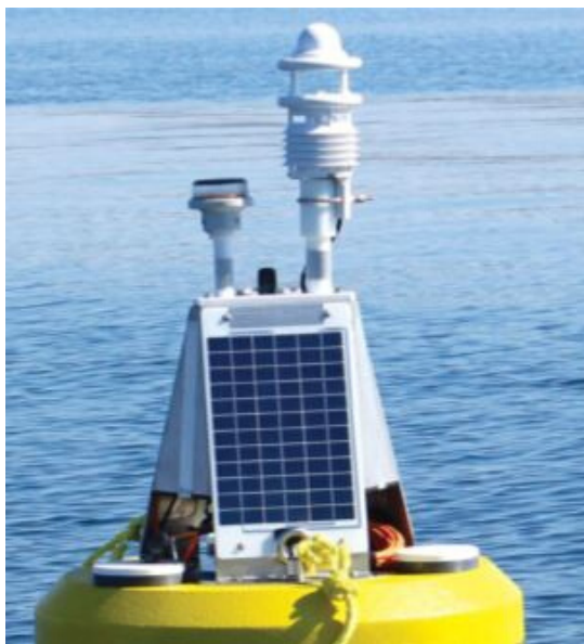
Image: The solar-powered buoy that will provide the platform for the monitoring station
