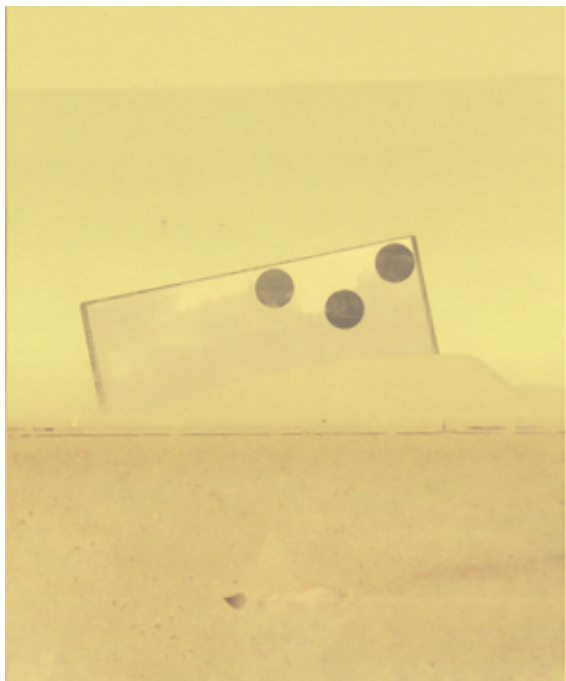
Image: Subsea structure settling due to scour on a mobile sediment bed.
